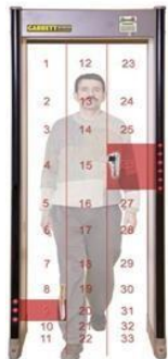
detection zones: 11 from top to bottom, using three separate zones to indicate later or right side of a patron.
